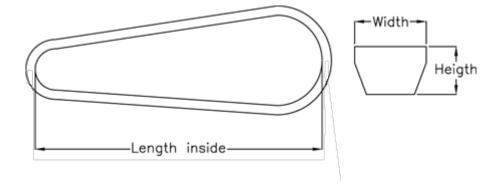
$\begin{array}{ll} \text{Datum Llength} = 6585 \\ \text{Height} & = 10 \\ \text{Length inside} & = 6545 \\ \text{Width} & = 17 \end{array}$
